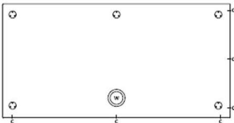
ON RECTANGULAR TRAYS, ENSURE THE PANEL CLIPS ARE FITTED TO THE SIDE REQUIRING PANELS. THIS IS DEPENDENT ON THE WASTE POSITION.
