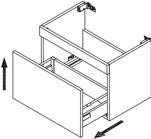
Remove drawer from cabinet prior to fitting unit to the wall. Pull-out the drawer to it's full extension and gently lift the drawer box upwards until it disengages from the runner.
