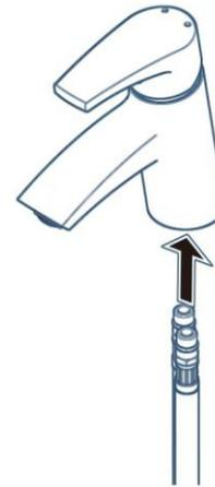
Screw the flexi / copper tails into the bottom of the mixer body by **hand only** (**DO NOT OVERTIGHTEN**)
