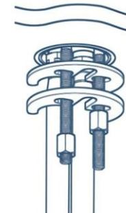
Slide the 'C' shaped rubber washer and the 'C' shaped metal washer onto the fixing rods up to the underside of the basin. To secure the mixer in place tighten the fixing nuts onto the fixing rods until they fully tightened against the 'C' shaped metal washer. A suitable spanner can be used to fully tighten the fixing nuts.
